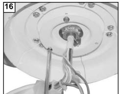
Loosen 2 screws with key slots and remove 1 screw without slot from motor plate and save screw.
